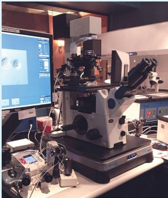
**Superior low frequency performance.** Starts to isolate at 0.7 Hz. Dramatic vibration cancellation, especially in the critical 1-10 Hz range.
